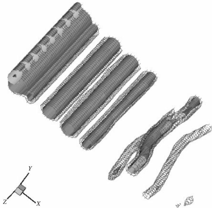
FIGURE 19. Rigidly moving cylinder at Re = 300 : pressure isocontours at values -0.3 and -0.4 . View facing the inflow from the side (flow is in the direction of the positive x -axis).
